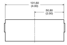
\* - 6,35 (0.25) O.D. tube G<sup>1</sup>/<sub>4</sub> (metric) .4375-20 UNF-2B thd. (inch) 2 places
