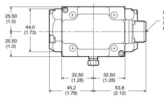
Electrical connector mates with MS-3106-14S-2S (4 pin). Plus signal to A or C causes flow out of port B.
